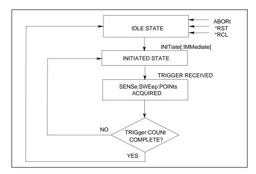
Figure 7-4. Model of Measurement Trigger System
